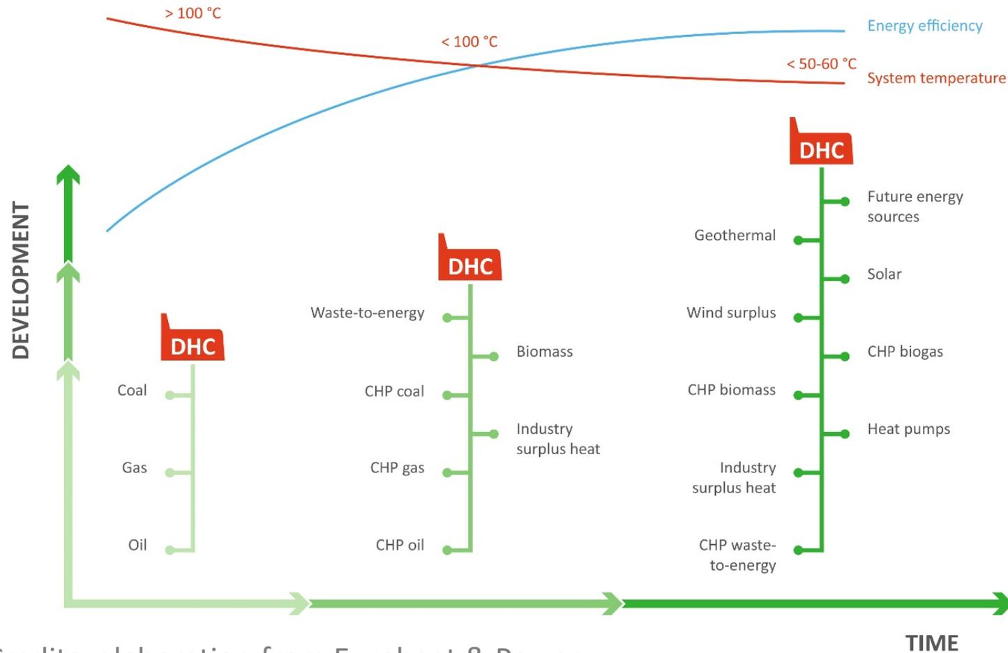
From fossil fuel based heating systems, to renewable based systems producing heat and power. Including thermal storage.
