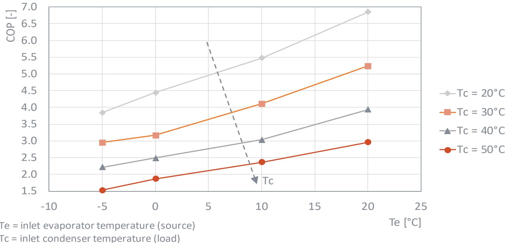
Example of COP variation of a heat pump in dependence of the inlet evaporator temperature. Shrinking temperatures lead to a shrinking COP. Eurac Research laboratory tests of a water / water heat pump with a nominal power 9.4 kW. Credits and further information Diego Menegon et. all, publications listed below
