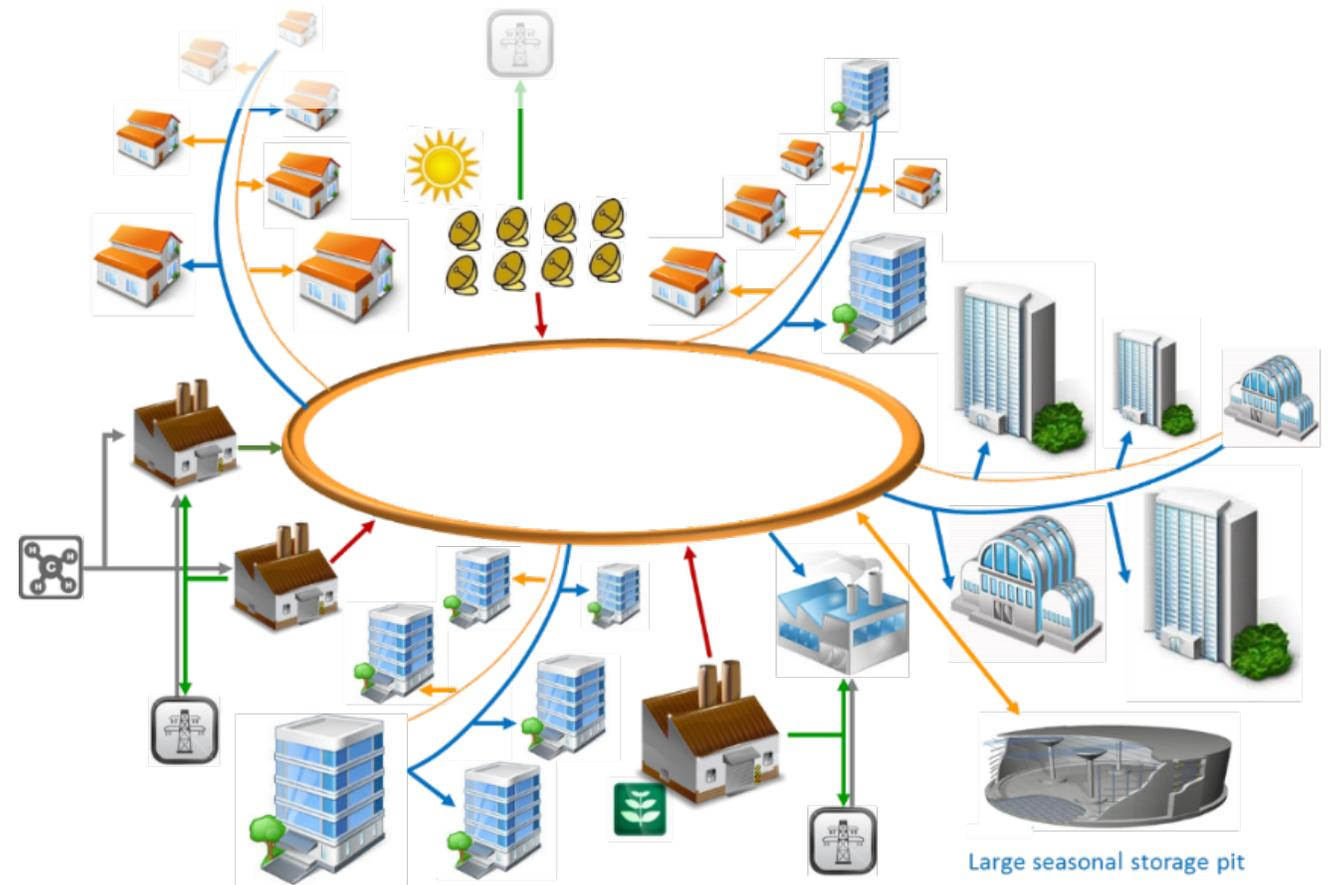
A decentralised low-temperature DHC network at  $15-25\text{ }^{\circ}\text{C}$  for new city quarters or grid expansion
