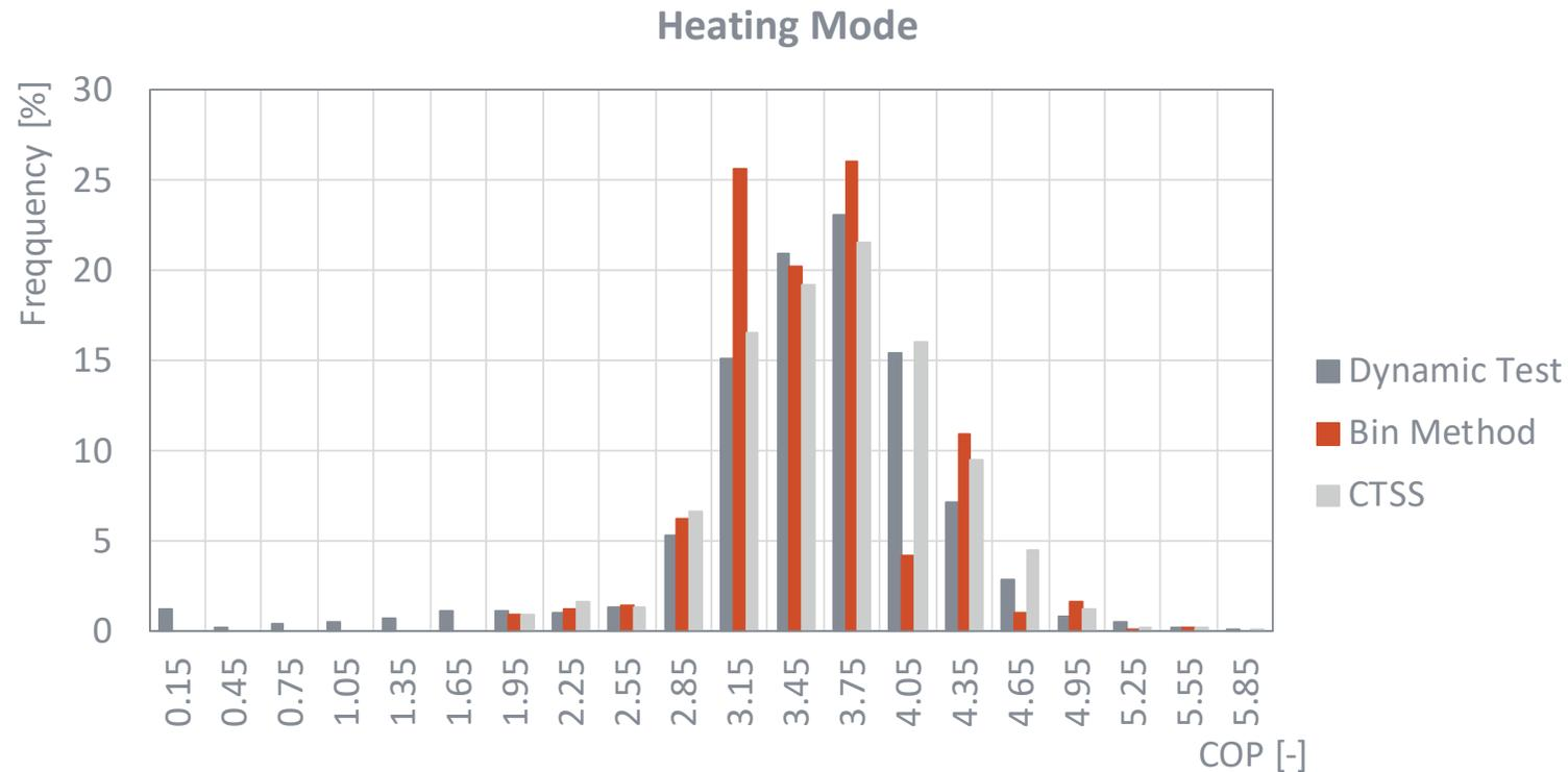
Frequency of presence of single COP values at the utilization of a heat pump over a full year.
