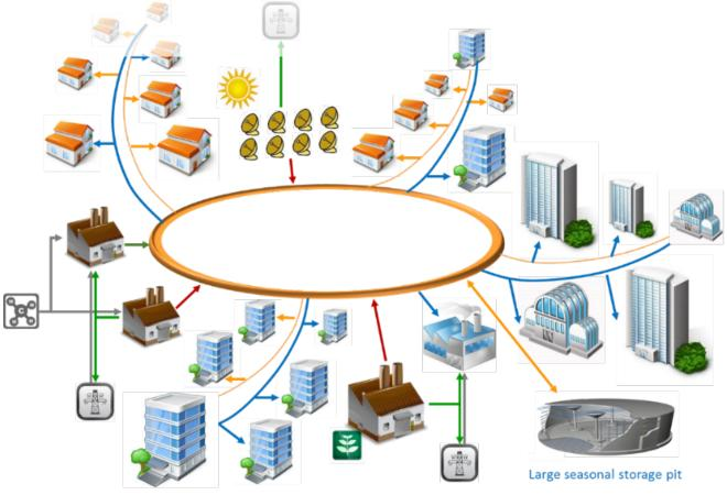
A decentralised low-temperature DHC network at 15-25 °C for new city quarters or grid expansion
