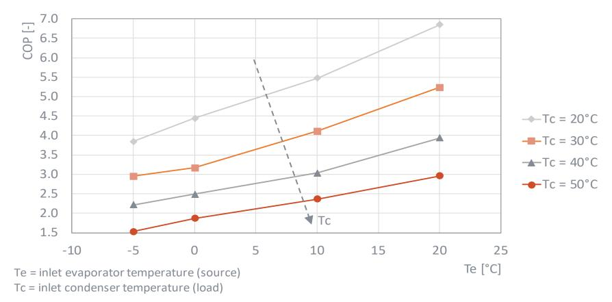
Example of COP variation of a heat pump in dependence of the inlet evaporator temperature. Shrinking temperatures lead to a shrinking COP. Eurac Research laboratory tests of a water / water heat pump with a nominal power 9.4 kW. Credits and further information Diego Menegon et. all, publications listed below
