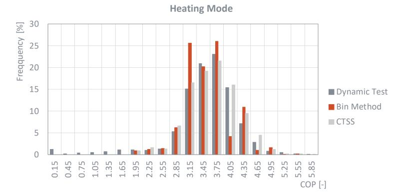
Frequency of presence of single COP values at the utilization of a heat pump over a full year. External climate data from Bolzano. Eurac Research laboratory test.
