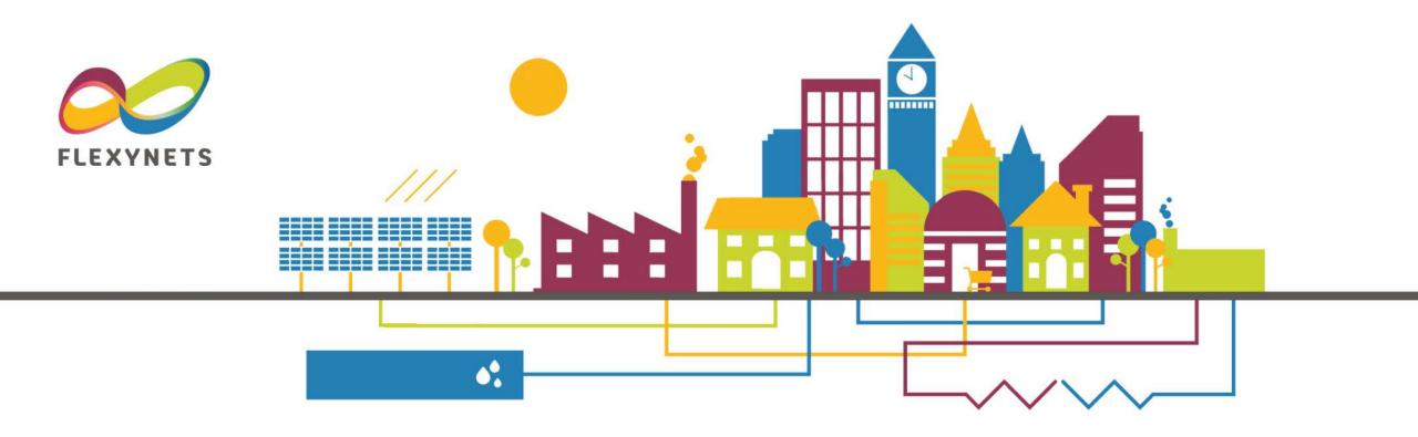
The traditional substations of district heating systems are replaced with heat pumps. End-users become prosumers in dependence of their energy needs. The heating network serves as well as low temperature storage.
