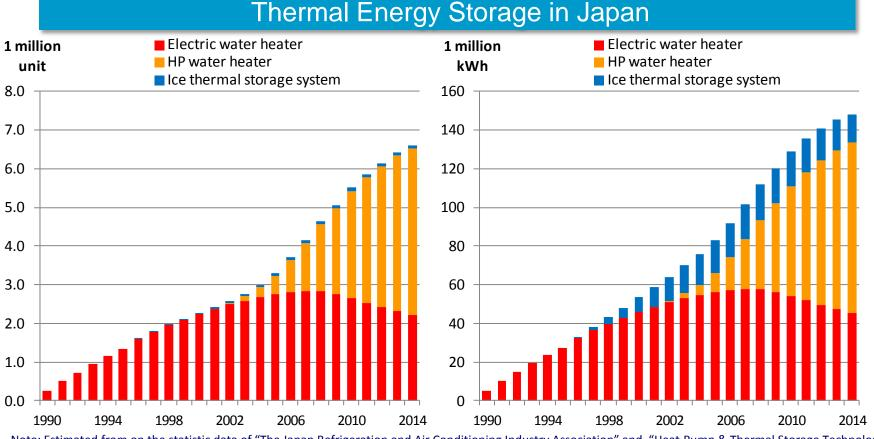
Note: Estimated from on the statistic data of "The Japan Refrigeration and Air Conditioning Industry Association" and "Heat Pump & Thermal Storage Technology Center of Japan". The annual shipment from this two data resources are used to estimate the penetration.
