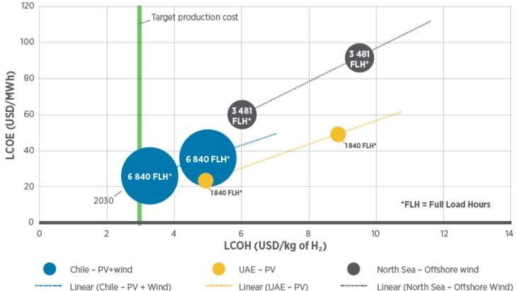
\* Bubble size proportional to load factor of electrolyser, depending on full load hours of VRE
