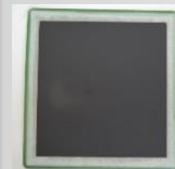
CEA Cell at the state of the art Characteristics Working point 1A/cm 2 Degradation 2-3% 1000h Active Surface 100cm 2
