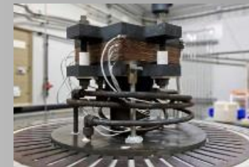
Electrolyzer core 25 cells Power 3kW
