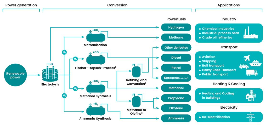
Includes: Fischer-Tropsch synthesis, hydrocracking, isomerization and distillation.
