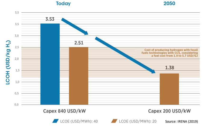
Key assumptions electrolyser: Load factor: 4200 hours (48%), conversion efficiency 65% (today), 75% (2050)
